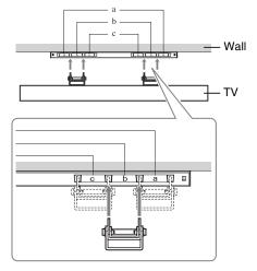
**2** Adjust the angle of the Mounting Hook.
